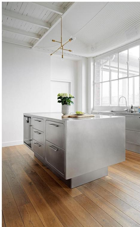
Above: Abimis uses extra-thick, scratch- and ding-resistant AISI 304 stainless steel and its worktops are fabricated from single sheets.
